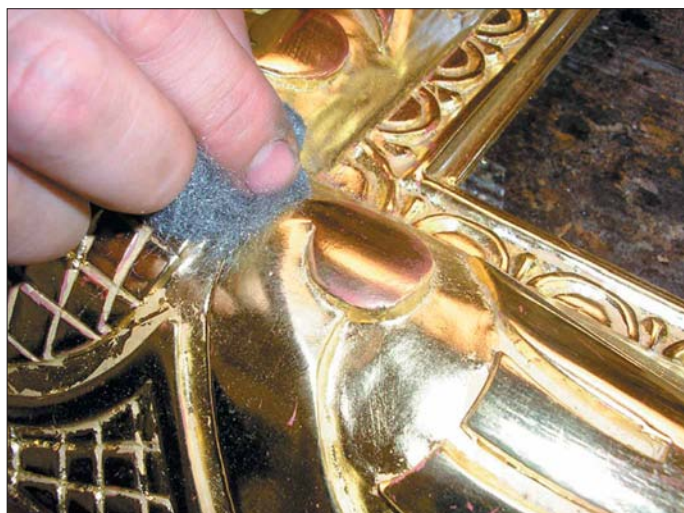
A light rub with very fine steel wool exposed some of the clay and added a look that resembled the effect that cleaning over time creates.
