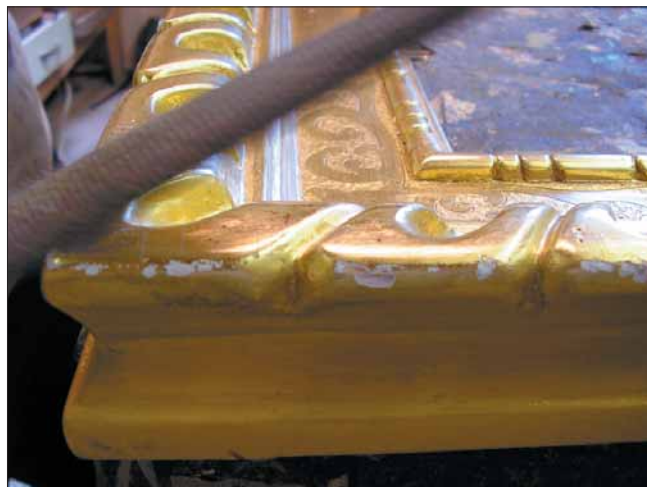
A rasp is used to make chips marked along the outside edge of the frame to replicate the dings a frame receives over time.
