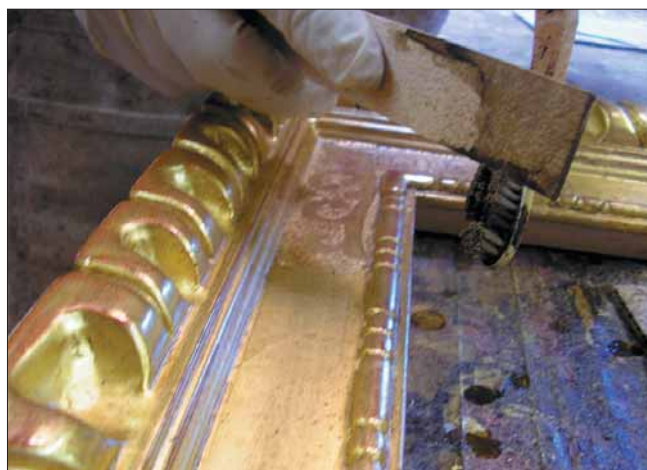
A toothbrush is used to add spatter. The brush carries the shellac and pigment mixture, and a wooden stick is drawn across the bristles to flick small droplets onto the frame.
