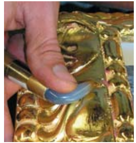
After that, the gilded frame is burnished to bring out the highlights of the profile.
