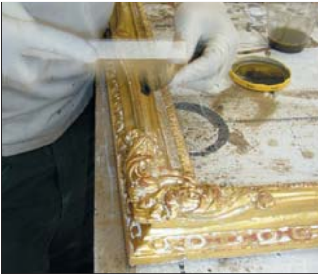
Next, the surface is spattered with raw umber artist pigment and clear shellac thinned with denatured alcohol.
